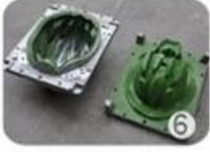
EPS in-mold tooling
