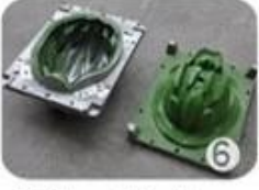
EPS in-mold tooling
