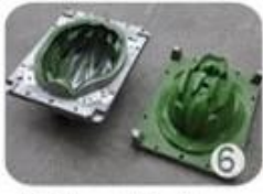
EPS in-mold tooling
