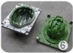
EPS in-mold tooling
