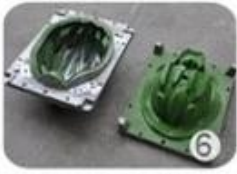
EPS in-mold tooling
