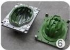
EPS in-mold tooling
