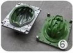
EPS in-mold tooling
