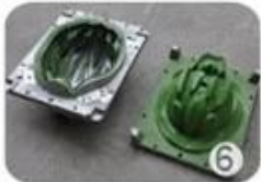
EPS in-mold tooling
