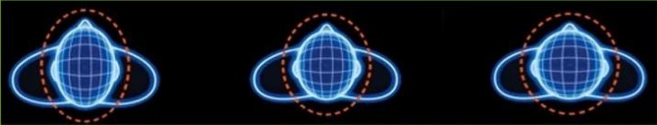
The image shows three wireframe head models on a black background, each with a blue grid and a red dashed oval representing the helmet shape. The first model is labeled 'European Headform' and shows an oval shape. The second is 'Generic headform' and shows a shape that is slightly longer front-to-back. The third is 'Asian headform' and shows a round shape.
