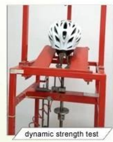
Shock Absorbing Capacity
