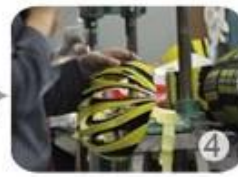
Trimming dug hole
