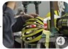
Trimming dug hole
