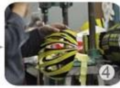
Trimming dug hole
