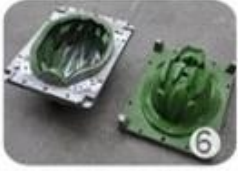
EPS in-mold tooling
