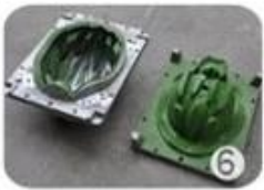
EPS in-mold tooling
