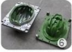
EPS in-mold tooling
