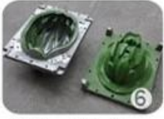
EPS in-mold tooling
