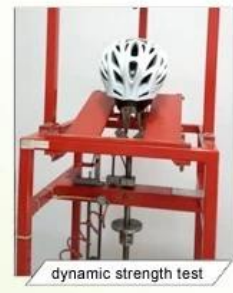
Shock Absorbing Capacity
