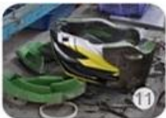
semi-finished In-mold helmet
