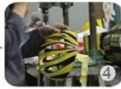
Trimming dug hole
