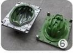
EPS in-mold tooling
