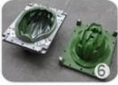
EPS in-mold tooling
