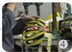
4 Trimming dug hole
