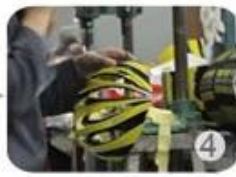
Trimming dug hole
