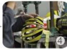
Trimming dug hole
