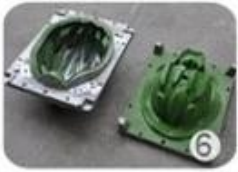
EPS in-mold tooling
