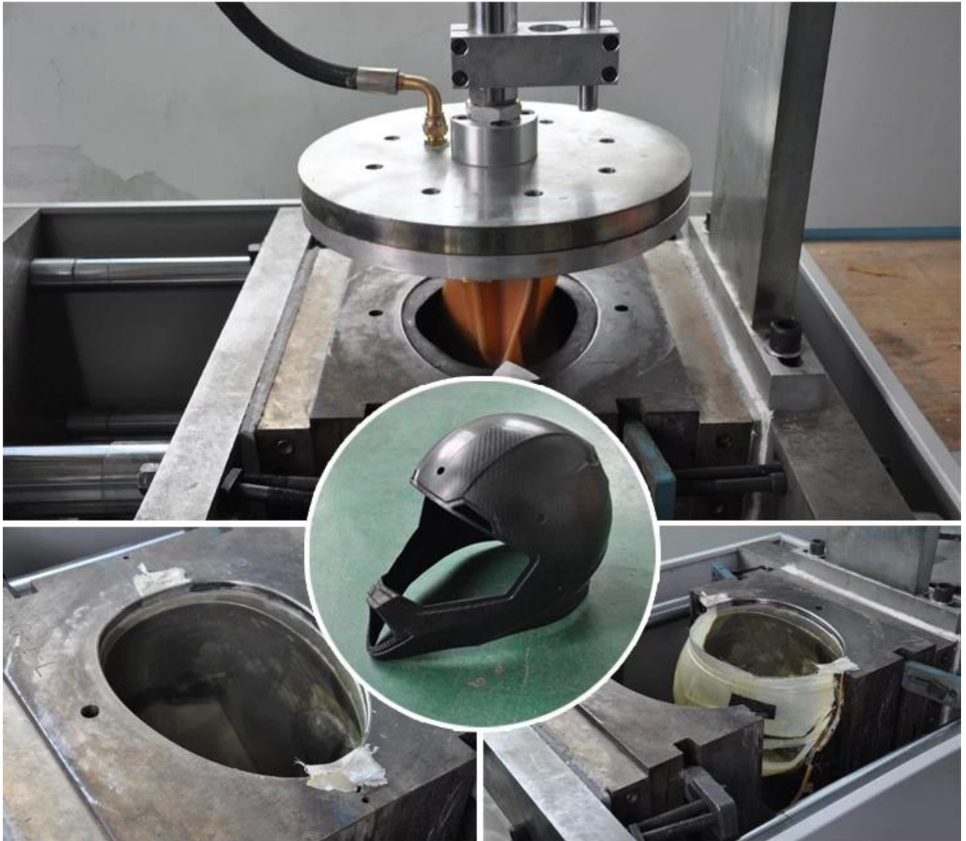
2. Autoclave Processing (Vacuum workach)
