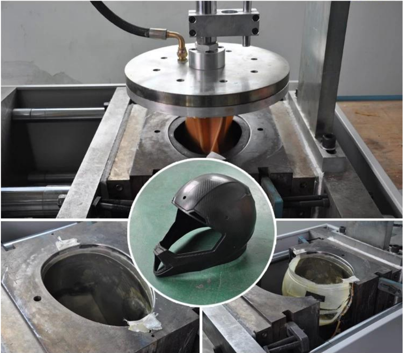
2. Autoklaw Processing (Vacuum workach)
