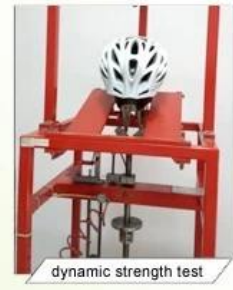
Shock Absorbing Capacity
