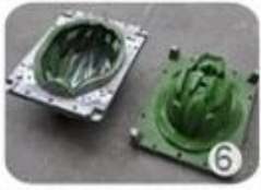
EPS in-mold tooling
