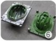
EPS in-mold tooling
