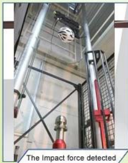
The Impact force detected
