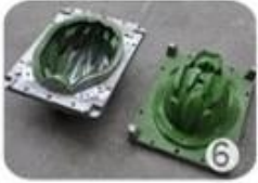
EPS in-mold tooling
