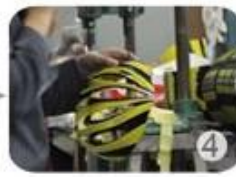
Trimming dug hole
