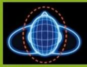
European Headform A long Oval shaped helmet is designed for a rider's head with a dimension which is considerably longer front-to-back than its side-to-side measurement.
