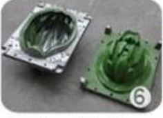
EPS in-mold tooling
