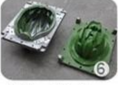
EPS in-mold tooling
