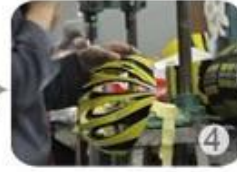
Trimming dug hole
