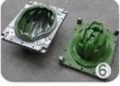
EPS in-mold tooling
