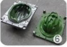
EPS in-mold tooling
